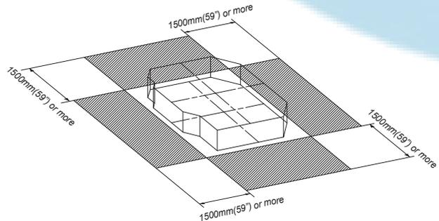
Proper clearance must be maintained around unit for proper operation.
